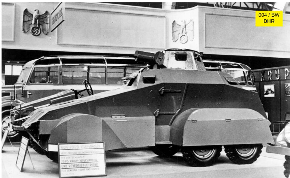
A number of German firms produced prototypes of armored cars for the police and the military. Here we see a Krupp *Polizei-Streifenwagen* displayed at an automobile show. The police patrol vehicle had a 70-horsepower engine and appeared to have the capability of mounting a machine gun in a revolving turret. The date and location are unknown. MICHAEL H. PRUETT
