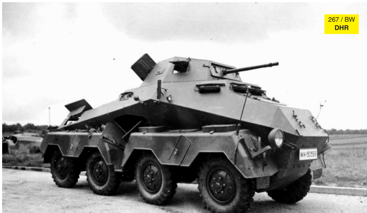
This Sd.Kfz. 231 (8 Rad) appears to be bereft of all basic-issue items. The relatively short staffs with the ball tops on the front sides of the vehicle are width indicators of the vehicle as an aid for the driver. JIM HALEY
